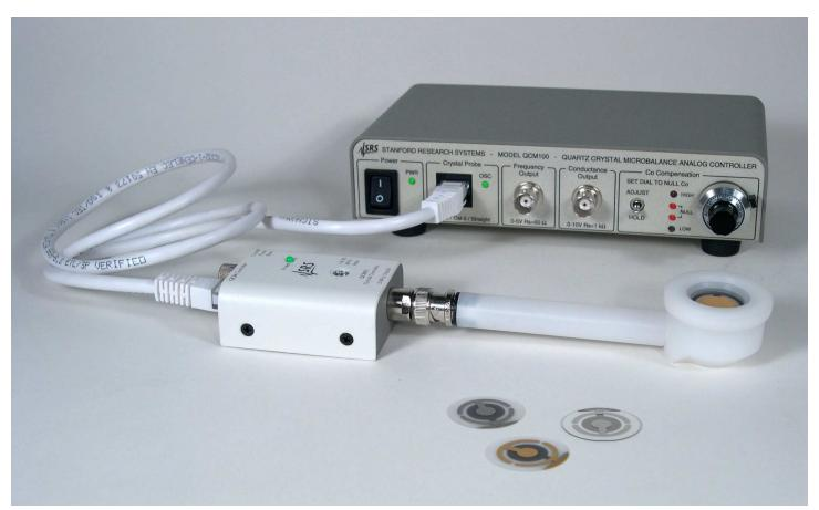
quartz crystal resonator with the necessary gain to overcome viscoelastic losses and achieve series resonance, while providing a signal that monitors the energy dissipated by the sensor (i.e. related to the series resonance resistance). The crystal oscillator will reliably drive crystals with resistance up to 5 k $\Omega$ . For example, it will maintain oscillation in viscous aqueous solutions containing over 88 % glycerol (w/w %).
